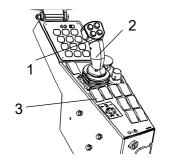
Fig. Control panel 1. Vibration On/Off switch 2. Forward/Reverse lever 3. Parking brake
