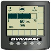
Fig. Compaction meter display (CMV display)
