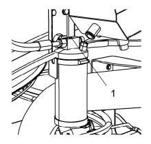
Fig. Drying filter 1. Sight glass
