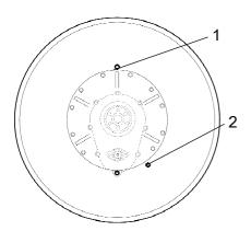
Fig. Drum, right side 1. Filler plug 2. Level glass If necessary, release the filler plug (1) and fill to half the sight glass (2).
