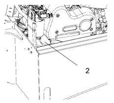
Fig. Engine compartment 2. Oil filter
