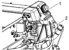
Fig. Expansion tank 1. Filler cap 2. Level indicator
