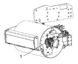
Fig. Oil filling - drum gear 1. Drum gear
