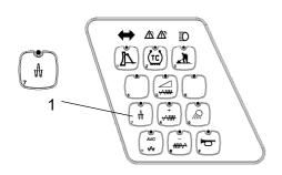
Fig. Control panel 1. High amplitude
