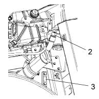
Fig. Hydraulic reservoir 2. Filler cap/Bleeding filter 3. Sight glass
