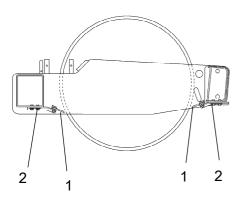
Fig. Scrapers 1. Scraper blade 2. Screws
