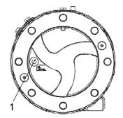
Fig. Level check - planetary gear 1. Level/Filler plug
