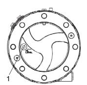
Fig. Level check - planetary gear 1. Level/Filler plug
