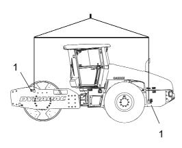
Fig. Roller prepared for lifting 1. Lifting plate
