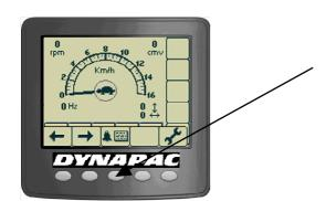
Alarms received are logged and can be seen by selecting Display alarms.
