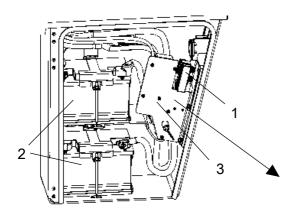
Fig. Cover, left side 1. Fuse box 2. Batteries (x2)
