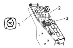
Fig. Control panel 1. TC (Anti-spin) 2. Forward/Reverse lever
