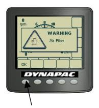
When a machine alarm is activated the alarm is shown on the display, plus a warning text that describes the alarm.
