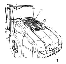
Fig. Engine hood 1. Hood lock 2. Protective grille
