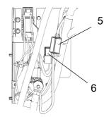
5. Fuse Engine-ECU(ECM) (F13), 30A 6. Fuel solenoid relay
