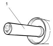
Fig. Air filter 1. Backup filter
