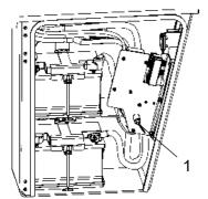
Fig. Cover, left side 1. Master switch
