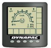
Fig. The display shows whether TC (Anti-Spin) is activated or disengaged
