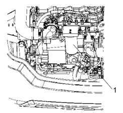
Fig. Engine compartment 1. Fuel filter
