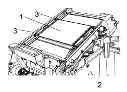
Fig. Engine compartment Condenser element
