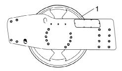
Fig. Left drum side 1. Groove
