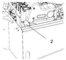
Fig. Engine compartment 2. Oil filter
