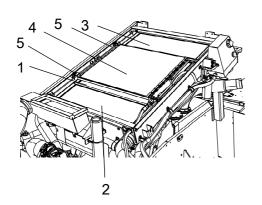
Fig. Engine compartment 1. Water cooler
