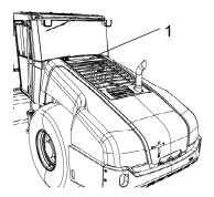
Fig. Engine compartment 1. Fuel filter
