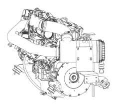
Check that the hose clamps between the filter housing and the suction hose are tight and that the hoses are intact. Inspect the entire hose system, all the way to the engine.
