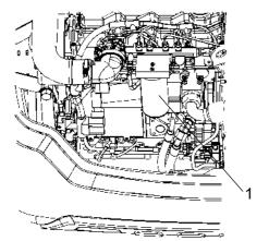
Fig. Engine compartment 1. Fuel filter
