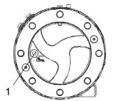
Fig. Planetary gear/filling position 1. Plug
