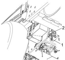
Fig. Machine's right underside 1. Drain cock 2. Plug
