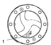
Fig. Planetary gear/drainage position 1. Plug
