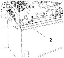
Fig. Engine compartment 2. Oil filter
