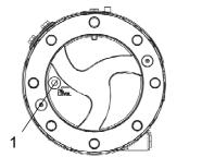
Fig. Planetary gear/filling position 1. Plug
