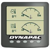
Fig. Temperature screen
