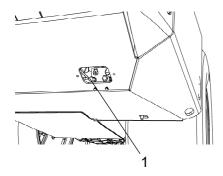
The oil drain plug (1) can be accessed most easily from the right rear underside of the tractor frame, and is installed with a hose in the engine.
