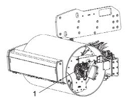
Fig. Oil filling - drum gear 1. Drum gear
