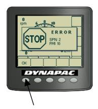
When an engine alarm is activated, the alarm is shown on the display.
