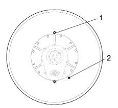
If necessary, release the filler plug (1) and fill to half the sight glass (2).
