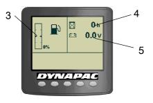
Fig. Status image 3. Fuel level 4. Hourmeter
