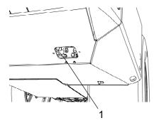
Fig. Tractor frame 1. Drain plug
