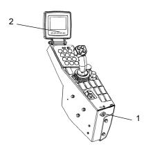
Fig. Control panel 1. Ignition key 2. Status screen
