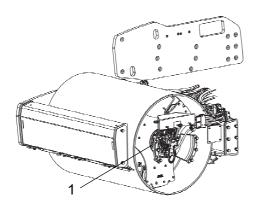
Fig. Checking the oil level - Drum gearbox 1. Drum gearbox
