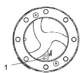
Fig. Planetary gear/drainage position 1. Plug
