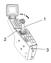
Fig. Control panel 1. F/R lever 2. Rpm switch 3. Ignition key
