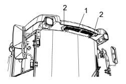
Fig. Cab 1. Fresh air filter (x 2) 2. Screws (x 3)
