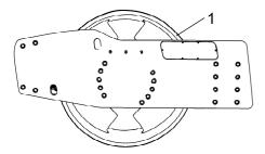
Fig. Left drum side 1. Groove
