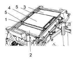
Fig. Engine compartment 1. Water cooler
