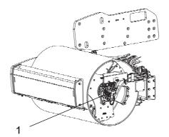
Fig. Oil change - drum gear 1. Drum gear
