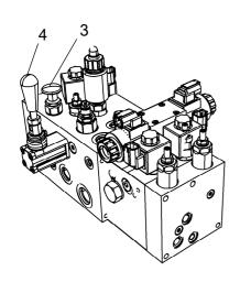
Fig. Valve block, engine compartment 3. Brake release button
