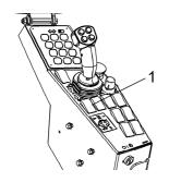
Fig. Control panel 1. Parking brake
