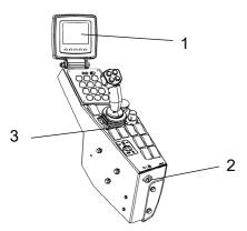
Fig. Control panel 1. Display 2. Ignition lock 3. Parking brake
