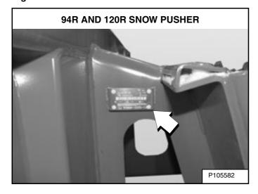
Always use the serial number of the snow pusher when requesting service information or when ordering parts. Earlier or later models (identification made by serial number) may use different parts, or it may be necessary to use a different procedure in doing a specific service operation [Figure 1] or [Figure 2].
