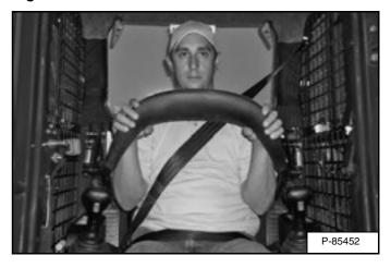
Lower the seat bar and engage the parking brake [Figure 17].
