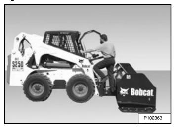
Use the snow pusher steps, grab handles (on cab) and the safety treads (on top of the loader lift arms and frame) to enter and exit the loader [Figure 15].
